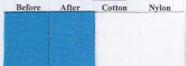
Sea Water Fastness Test (37±2°C X4hours)
