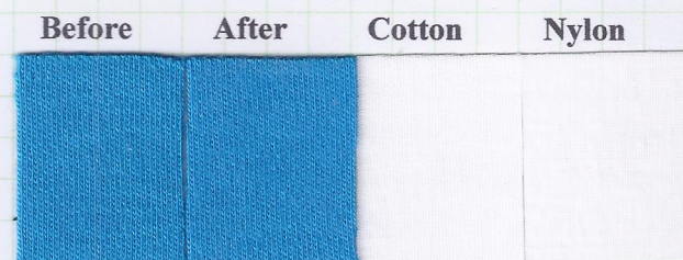
Light Fastness Test 40 hours
