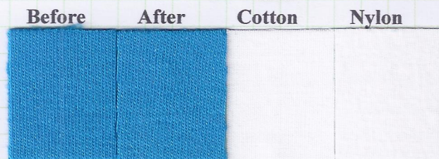
Water Fastness Test (37±2°C X4hours)
