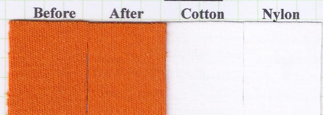
Sea Water Fastness Test (37±2°C X 4 hours)
