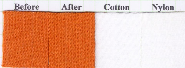
Water Fastness Test (37±2°C X 4 hours)
