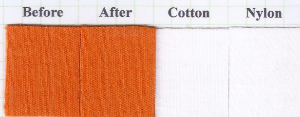
Light Fastness Test 40 hours
